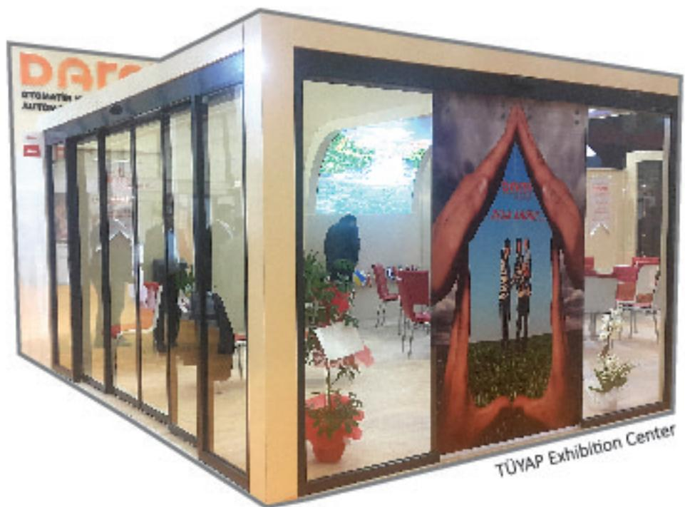
**Automated telescopic door system is the ideal system for narrow entrances. Sliding wings slide over each other with relative speeds in this system. Telescopic doors eliminate the passage space problem thanks to wings sliding over each other, whereas other automated door systems cannot provide the required passage space.**
